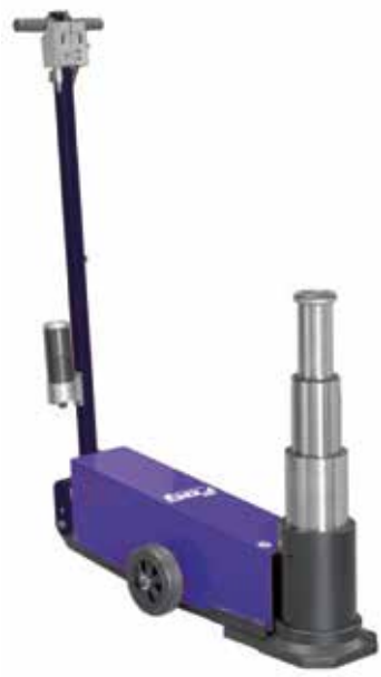
25T, 50T, 80T jack - 300/825 mm lifting height, 3 cylinder stages 163 9076
